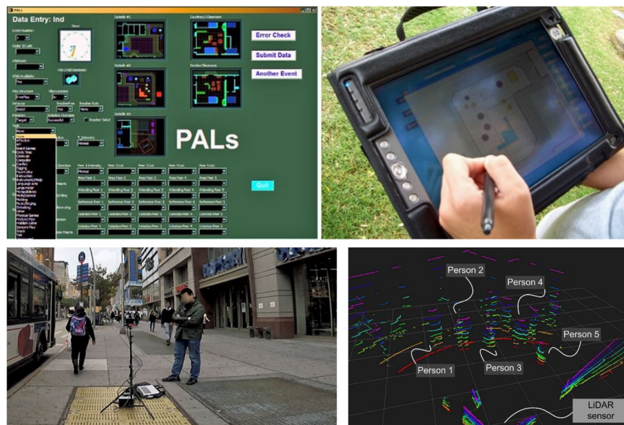
Fig. 3 Top: hand-coded labelling of motion parameters in real-world settings. Bottom: LiDAR measurement of spacings and timings in busy motion scenes
